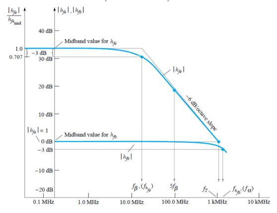
The frequency at which  $|h_{fe}|_{dB} = 0$  dB is clearly indicated by  $f_T$  in Fig. above. The magnitude of  $h_{fe}$  at the defined condition point  $(f_T \gg f_\beta)$  is given by
