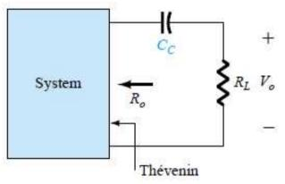
The cutoff frequency due to Cc is determined by:  $\frac{1}{2\pi(R_L+R_O)C_C}$
