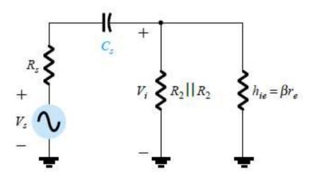
$$R_i = R_1 ||R_2|| \beta r_e$$
