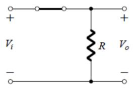
and the short-circuit equivalent can be substituted for the capacitor. The result is that  $V_o \cong V_i$  at high frequencies.
