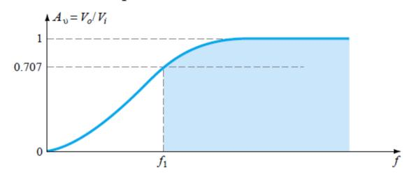
The output and input voltages are related by the voltage-divider rule in the following manner:
