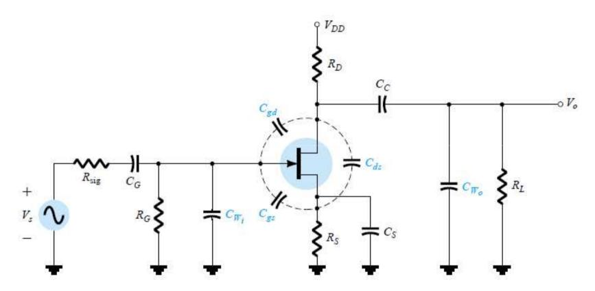
The cutoff frequencies defined by the input and output circuits can be obtained by first finding the Thévenin equivalent circuits for each section
