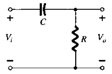
Our analysis, therefore, will begin with the series *R-C* combination of Fig. 11.8 and the development of a procedure that will result in a plot of the frequency response with a minimum of time and effort.
