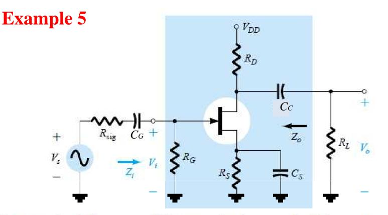
(a) Determine the lower cutoff frequency for **following network** using the following parameters:
