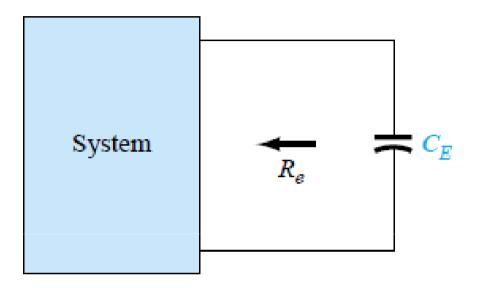
Once the level of  $R_e$  is established, the cutoff frequency due to  $C_E$  can be determined using the following equation:
