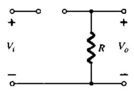
and the open-circuit approximation can be applied with the result that  $V_o = 0 \text{ V}$ .
